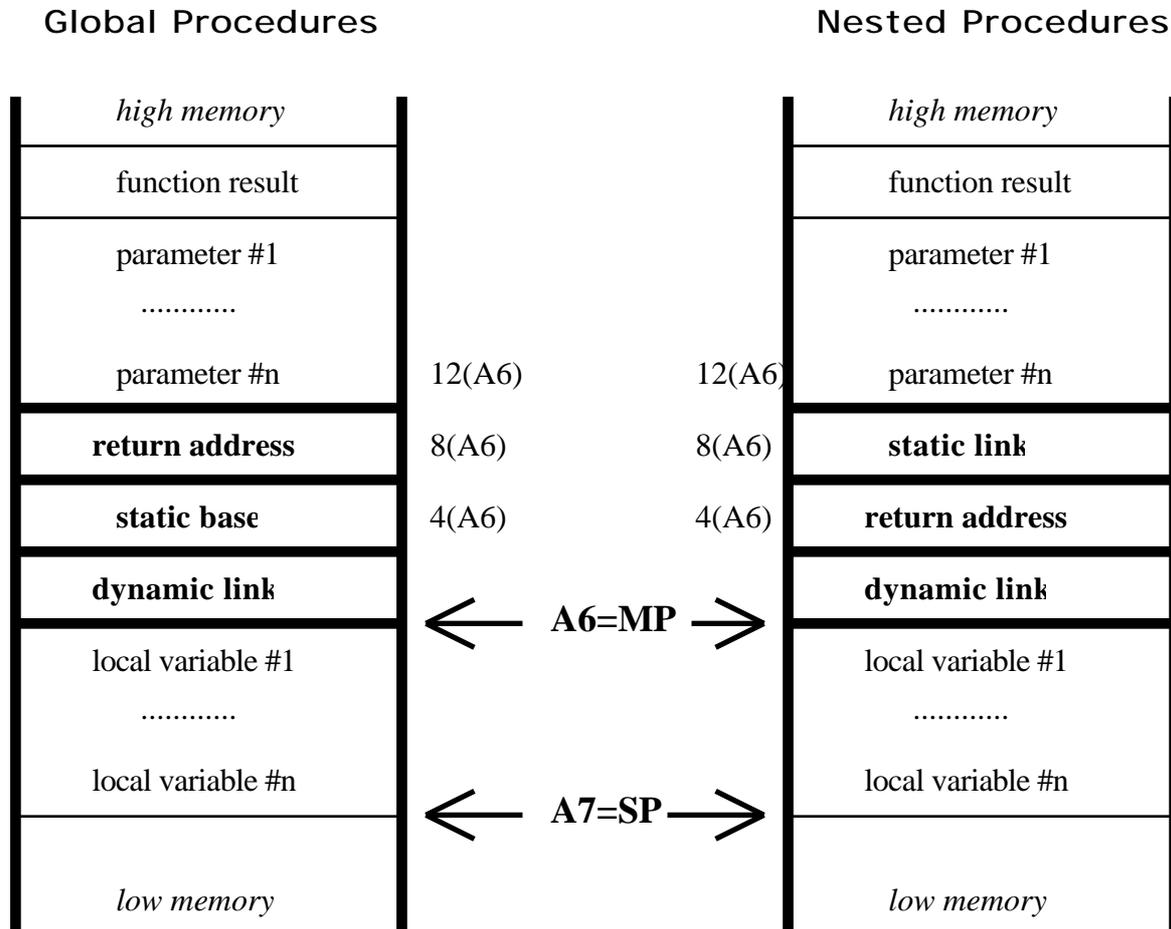
Fig. 4.7: System Stack and Procedure Mark
