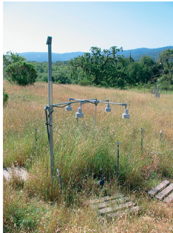
Fig. 3.5. An experimental plot in the Jasper Ridge Global Change Experiment. Four infrared heat lamps suspended over the 2-m diameter plot increase the canopy temperature by ~1 °C. Pure CO 2 is released from a circle of tubing surrounding the plot, enriching the CO 2 concentration in the air by about 300 ppm. Subplots comprise different combinations of precipitation and N deposition
