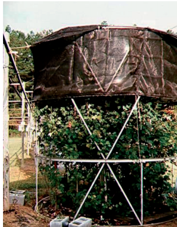
Fig. 3.3. Acer saccharum and A. rubrum trees in an open-top chamber at the conclusion of the TACIT experiment. The plastic panels of the chambers and lower portions of the shade cloth, which were present throughout the four growing seasons of the experiment, have been removed to facilitate harvesting of the trees
